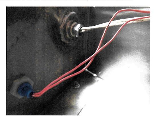
4. Use the box wrench to remove the fire rod from the water tank.
