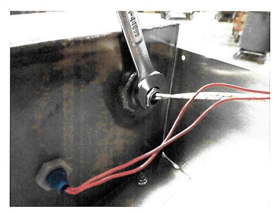
5. Then insert and tighten down new fire rod. Using the supplied wire nuts to wire nut together the ends of the exposed wires. It does not matter which wire goes where.
