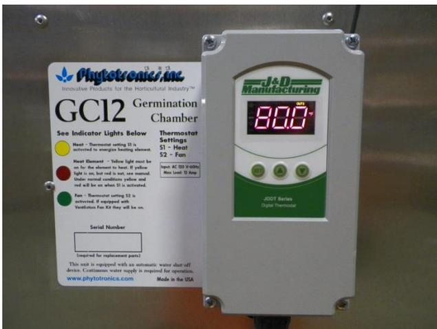
To change the fan activation temperature, Press “SET” 2X from “run mode”. OUT2 will be on the top edge of the display and the number will slowly blink. Factory set at 80. The arrow keys are used to raise or lower this number. Once the desired temperature is set then push “SET” once to enter “run mode” *for example at 80 the unit will need to reach an internal temperature of over 82 for the fans to come on and if cool enough outside then they will pull it back to 80 before they will turn off.*
