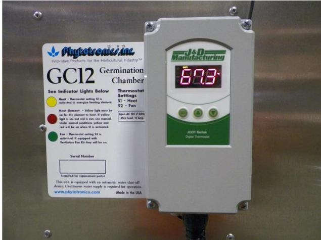
Plug Germination Chamber into outlet. The Thermostat will go through a startup cycle then show the internal temperature on the display in Fahrenheit. This is the “run mode” display. *On the top edge of the display when activated will be an OUT1 or OUT2. If OUT1 is displayed then the yellow & red lights and the heater below will be on. ( if only the yellow light comes on check water level in reservoir) If OUT2 is displayed then the green light below will be on, along with fans ( if equipped ).*
