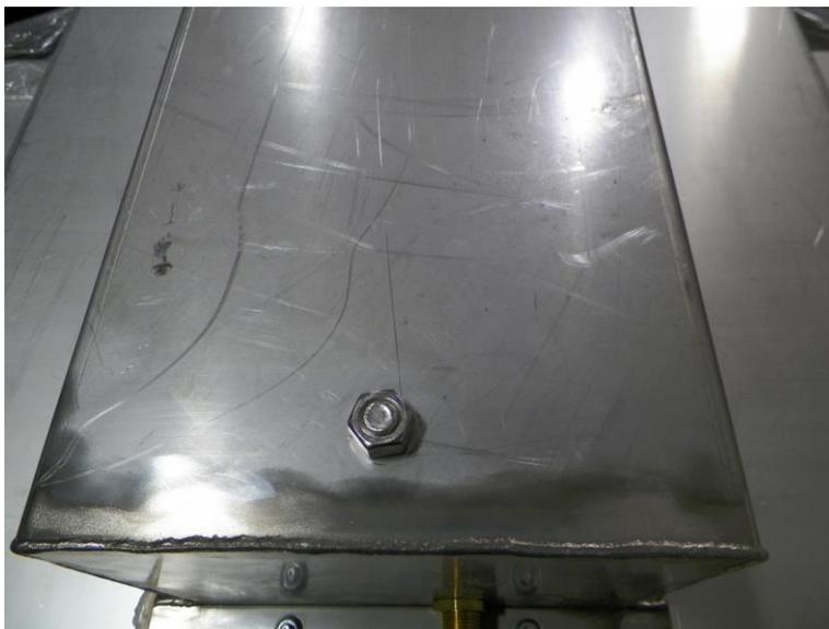
7. After the water has been drained. Dry the interior of tank with a towel. Reinstall the drain bolt. Be sure to place the washer back in.
