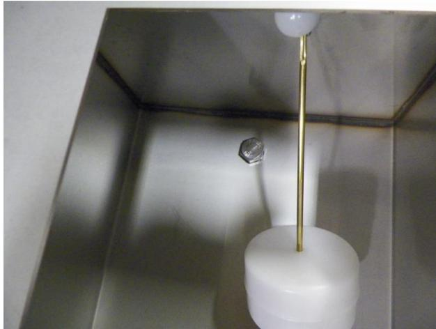
6. Locate the drain nut on the bottom side of the tank.
