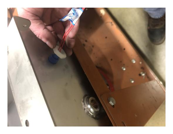
Replace the plastic wire nut to hold the switch in place. Nut is attached on the outside of the reservoir.
