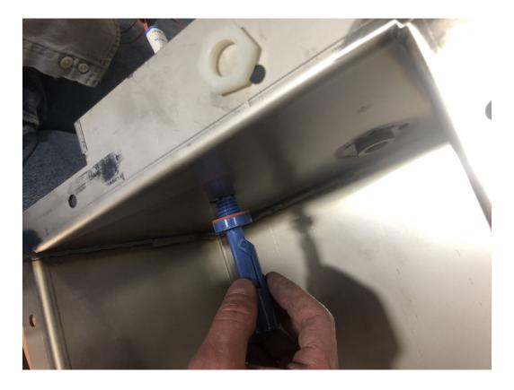
Remove the defective switch.
