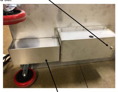
Lay Germination Chamber on its side. Remove 7 Phillips head screws that hold the electrical box cover in place.
