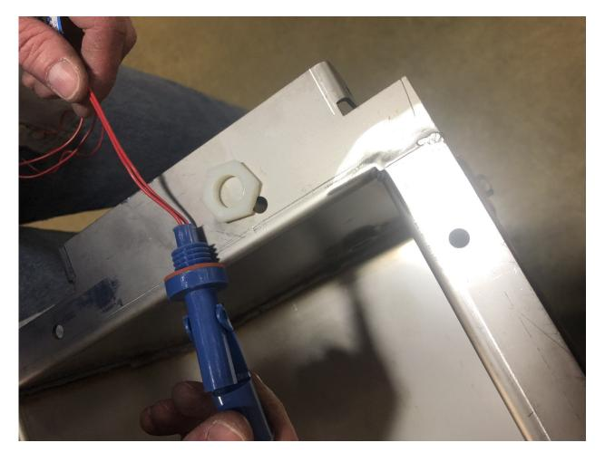
Insert the new float switch inside the reservoir, pulling the 2 wires through the wall and to the outside of the reservoir.
