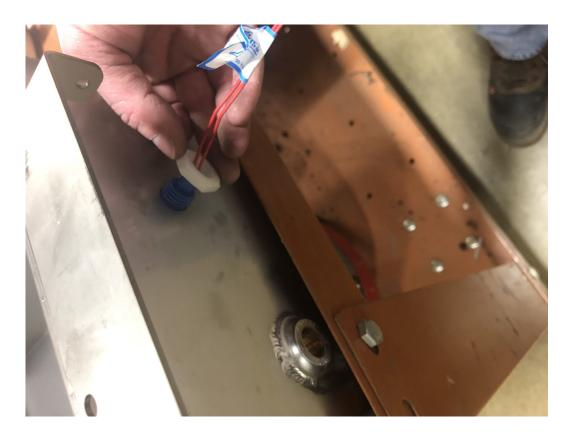
Unscrew the plastic nut on the outside of the reservoir that holds the float switch in place
