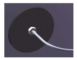
Locate the Pressure Adapter at least 5 feet from the Blower discharge as air turbulence will cause inaccurate pressure measurements. Clean and dry the surface of the selected location. Cut a small hole approximately 1/2" to allow the threaded part of the hose barb to enter the Inflation Chamber. Peal off the adhesive protective film and press the disc in place while centering hose barb in the hole in the Inflation Chamber. Extra tape maybe applied if necessary.
